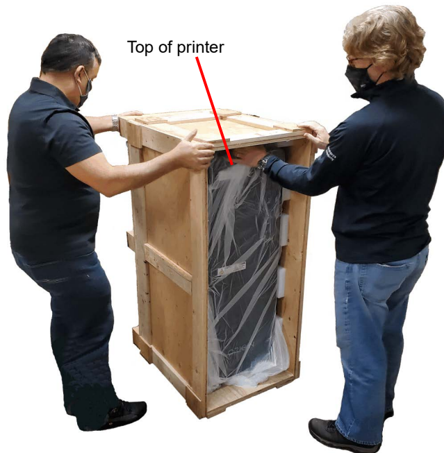
Figure 9: Standing the Shipping Crate
