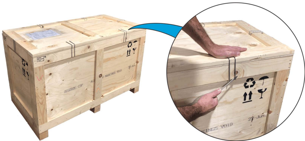
Figure 7: Removing the Shipping Crate Top Panel
